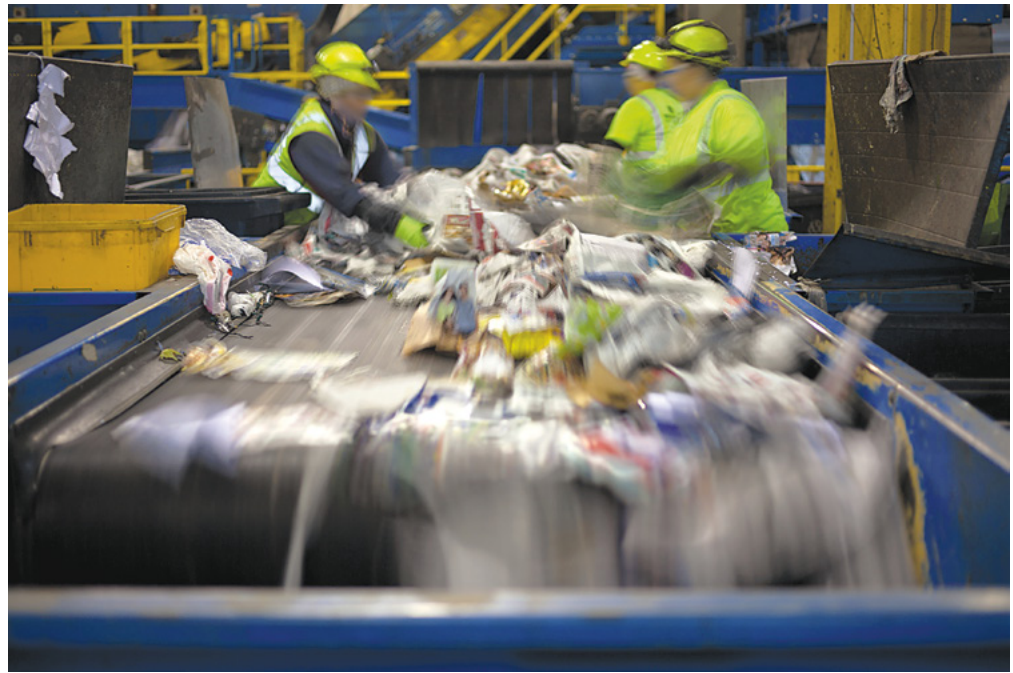
Workers pull recyclables off a moving conveyor belt in a recycling sorting facility. Materials coming into this facility come in as mixed recyclables from "single-stream" carts and bins.
